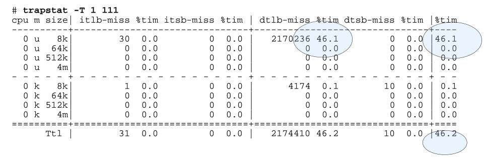
This application **could** potentially run 2x faster using large pages!
