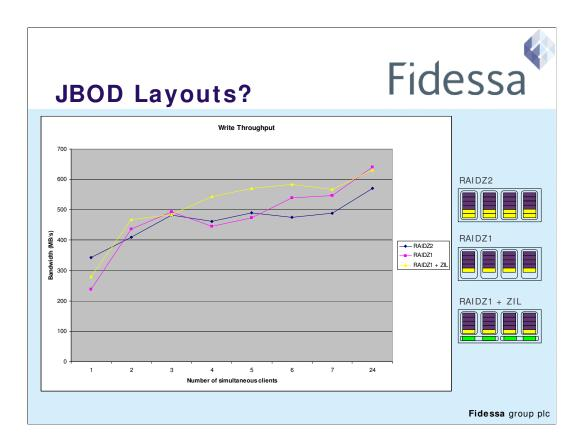
Here we have a graph of our measured bandwidth for writes during the rsync process against the number of hosts running simultaneously. It's linear up to 7 simultaneous hosts, but as this was showing a plateau effect, we took the next step as all our 24 test hosts at once.
