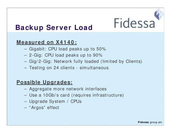
Our backup server for the proof of concept was an X4140 with 2 quad-core CPUs running at 2300MHz. We tried our runs on both a single gigabit connection and on two aggregated connections providing us with 2 Gbps.
