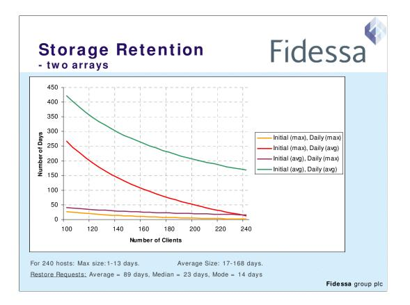
This graph shows 4 different choices depending on whether we use the maximum amount recorded or the average amount recorded for either of the initial full sync or the daily incremental sync. This is all calculated on two J4400 arrays which gives us about 28 TB of storage.
