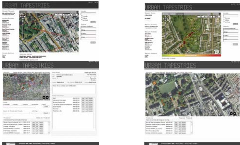
Figure 4. Urban Tapestries web interface: (a) browsing threads, (b) air quality sensor visualisation from RFFA, (c) creating pockets and threads, and (d) searching for pockets.
