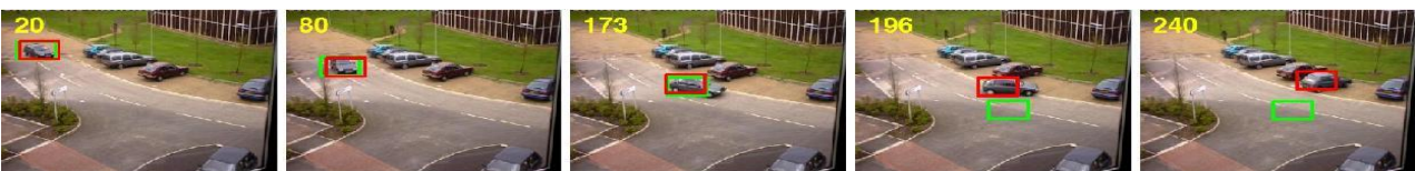
Fig. 4. The results of tracking a car which undergoes large changes in scale and appearance.
