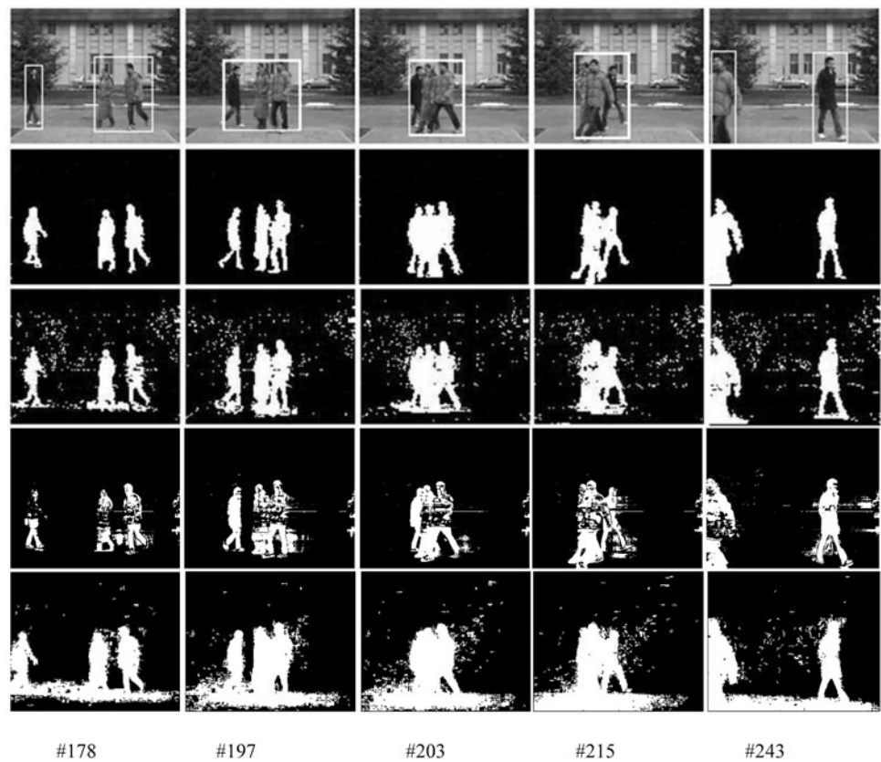
Fig. 8 Foreground segmentation for the second video: In row 1, the moving regions are highlighted by white boxes ; Rows 2, 3, 4, and 5 show the results of our algorithm, the original version of the vector subspace-based algorithm, the modified version of the vector subspace-based algorithm, and the GMM-based algorithm, respectively
