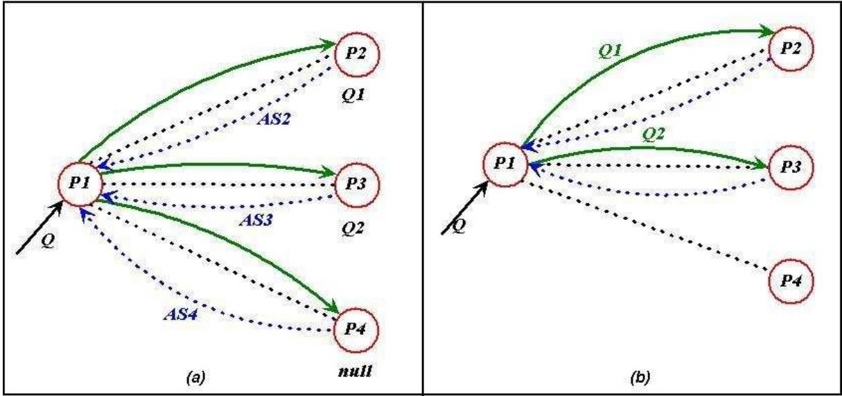
Figure 12: SQPeer Query Processing Mechanism in an Ad-Hoc P2P System
