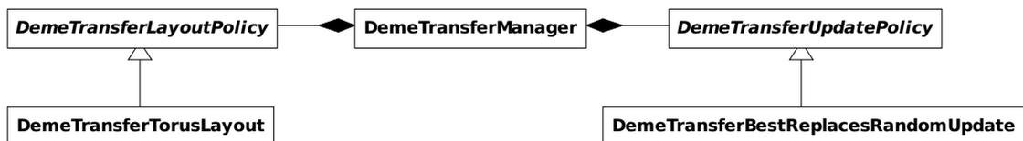
**Figure 34:** The `DemeTransferManager` class owns a `DemeTransferLayoutPolicy` and a `DemeTransferUpdatePolicy`. These two classes are abstract base classes with concrete instantiations such as `DemeTransferTorusLayout` and `DemeTransferBestReplacesRandomUpdate` respectively.
