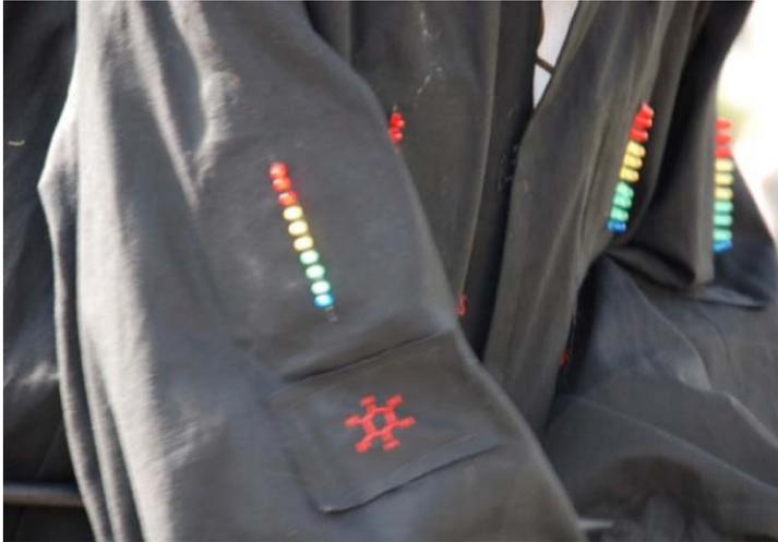
Wearable technologies developed at the London Knowledge Lab: Carnival performance costumes with embedded environmental sensing capabilities that display the current levels of various pollutants via LEDs sewn into the garments.
