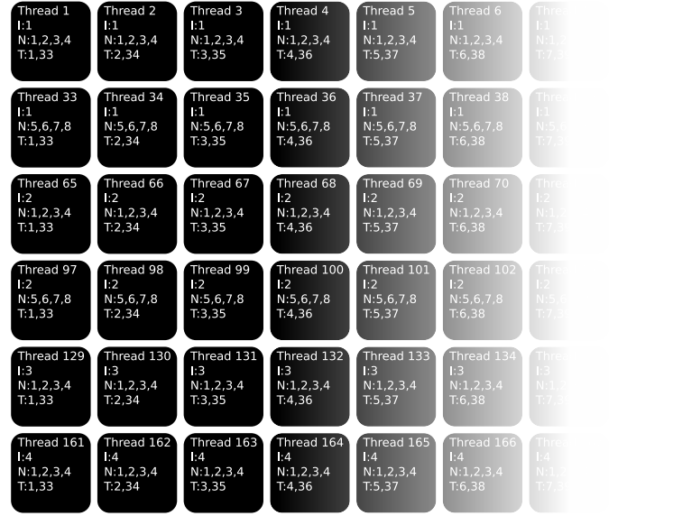
Figure 1: An example of the division of work in a block of 192 CUDA threads. The letter I precedes the individual’s number, N precedes the nodes’ numbers and T precedes the test cases’ numbers. Not all of the nodes are displayed as indicated by the fade to white.
