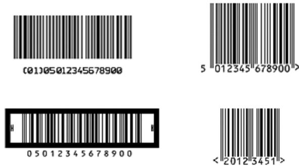
**Fig. 2.3.** Clockwise from the top left: samples of UCC/EAN-128, EAN-13, EAN-8, ITF 14.
