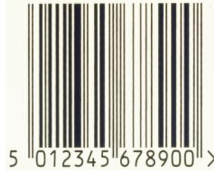
**Fig. 2.1.** A typical example of an EAN-13 bar code.
