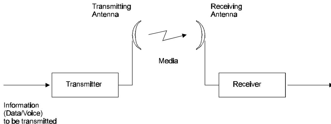
**Figure 1: A Typical Radio System**
