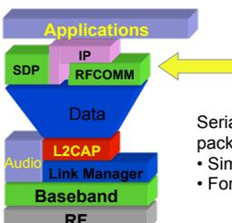
Serial Port emulation on top of a packet oriented link
