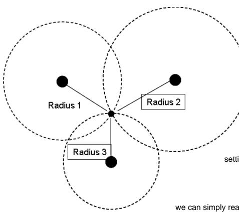
$$\begin{split} r_1^2 &= x^2 + y^2 + z^2 \\ r_2^2 &= (x-d)^2 + y^2 + z^2, \\ r_3^2 &= (x-i)^2 + (y-j)^2 + z^2 \end{split}$$
