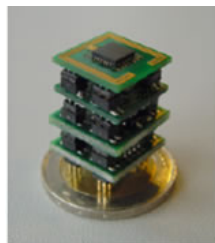
Fig. 1 The four layers of the IMEC Sensor Cube hardware platform. A 2€ coin provides a size reference.
