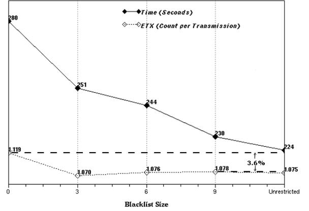
Fig. 1. The average length of time required to complete the transmissions of all packets (solid line with filled diamonds) tends to be shorter when blacklisting (non-zero blacklist size) is used. Blacklisting also makes average Expected Transmission Count (dashed line with hollow diamonds) at least 3.6% lower, indicating a better chance of successful transmissions.
