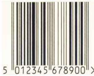
Fig. 2. A typical example of an EAN-13 bar code.
