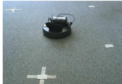
Fig. 3. iRobot Roomba with surrogate Shared Memories capture device. Also visible are the RFID tags forming a proximity detection grid on the floor.
