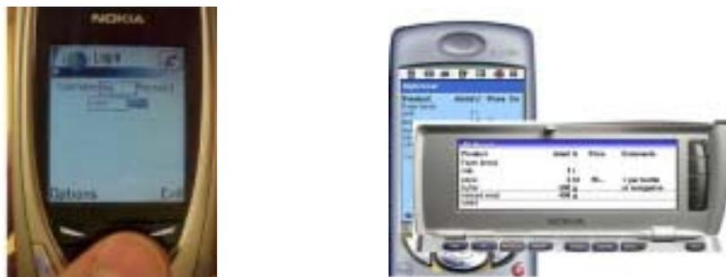
Figure 2: Access to retail m-services via cellular wireless mobile devices: user authentication (left) and shopping list editing (right) on wireless enabled personal digital assistant and cellular mobile telephone (both Java 2 Micro Edition capable).
