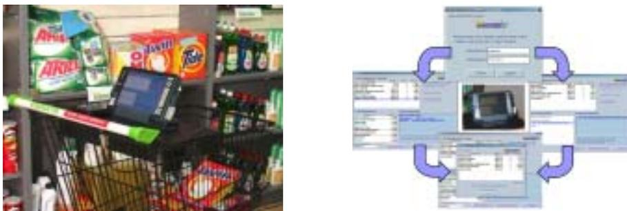
Figure 1: Prototype shopping cart implementation: Shopping cart with tablet PC, wireless network and RFID reader (left). User Interface: Login screen, shopping options including shopping cart content monitor, shopping list, total shopping cart content cost, offers and personalized promotions, additional product information and finally, fast check-out (right).
