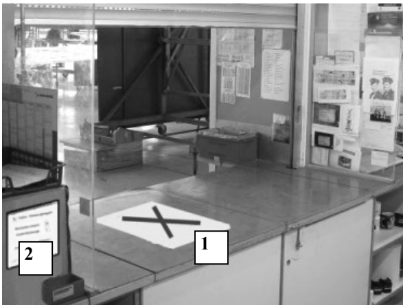
Fig. 3. Smart Tool Inventory setting with RFID reader and antenna (No. 1) and display (No. 2)
