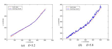
Fig. 11. Comparison: (a) Trajectory acquired using our method and true data. (b) Centroid trajectory and true data.
