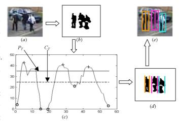
Fig. 4. Detection of principal axes of people in a group: (a) Input image. (b) Detected foreground region. (c) Vertical projection histogram. (d) Segmented individuals. (e) Principal axes.
