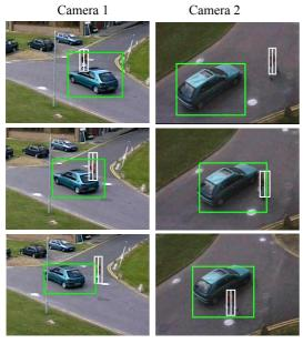
Fig. 8. Tracking and correspondence of a person occluded by a vehicle with two cameras: From the top to the bottom, the frame numbers are respectively 560, 578, and 590.
