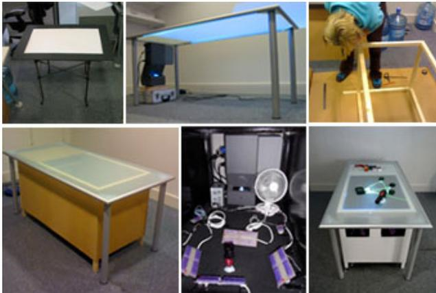
**Figure 1. Iterative development of the tangible table. Paper frame and camping table (top left); Sanyo PLC projector and IKEA table (top middle); constructing the housing (top right); final prototype (bottom left); interior including camera and IR LEDs (bottom middle); final design running the light scenarios in Processing (bottom right).**
