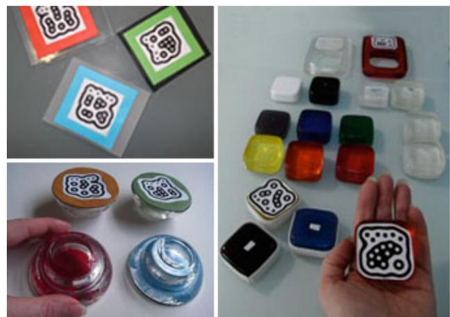
Figure 5. Iterative development of tangible artefacts with printed fiducials. Perspex and paper (top left); glass and leather (bottom left); crystal resin (right).
