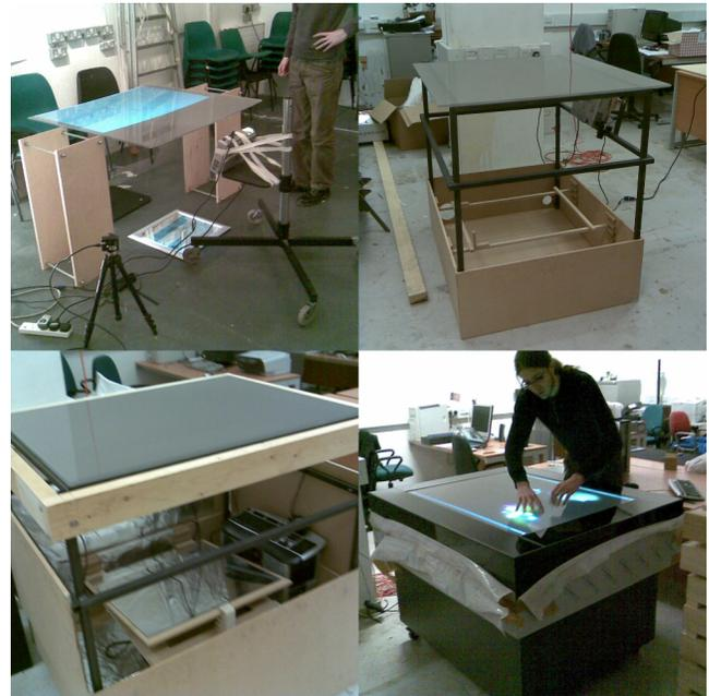
**Figure 2: Clockwise from top right: initial experiment (camera not correctly placed); steel frame, surface material and projector/camera mount; mirror and housing (foil was not used in final version); testing the nearly complete table with wide bezel top.**
