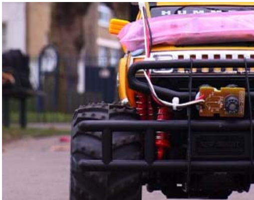
Figure 1. The prototype mobile sensor network node with carbon dioxide and air quality sensors.
