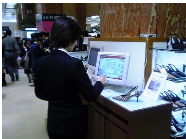
Fig. 3 Using a kiosk terminal in the shoe floor for women: When a shoe is placed on the table, the system automatically reads the RFID tag that is attached to it and shows relevant stock levels
