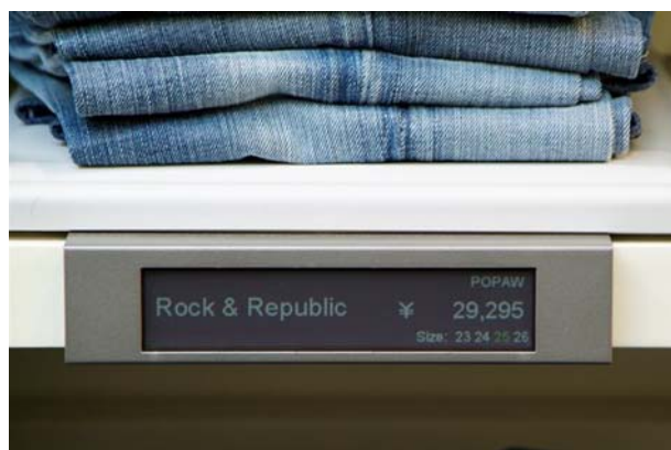
Fig. 4 Smart shelf showing the stock status on a color electronic paper display. RFID readers are embedded in the shelf to monitor the presence of jeans. White numbers indicate sizes that are available on the shelf. Green numbers indicate sizes that are not available on the shelf but available in the stockroom. Sizes that are unavailable are not shown
