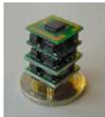
Fig. 1 The four layers of the IMEC Sensor Cube hardware platform. A 2Euro coin provides a size reference.
