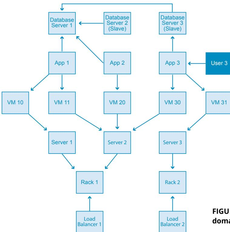
**FIGURE 3.1: A sample model of a data center management domain in its initial “whiteboard” form.**
