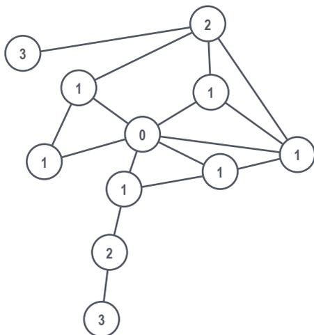
**FIGURE 8.1: An example path of a breadth-first algorithm, where the search begins at the node marked "0" and then traverses first to every node marked "1" before journeying on to nodes marked "2" and then finally visiting all nodes marked "3."**
