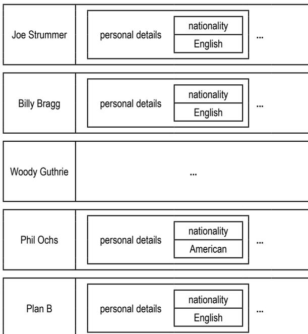
**FIGURE 11.5: Keys form a natural index through rows in a column family database.**
