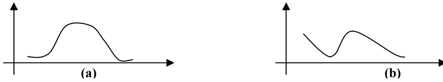
Figure 4. Uni-modal distribution shape on (a) versus a bi-modal distribution shape on (b): the standard deviation of the latter is greater, thus making the latter less significant under the z-scoring standardization, which is odd in the clustering context.
